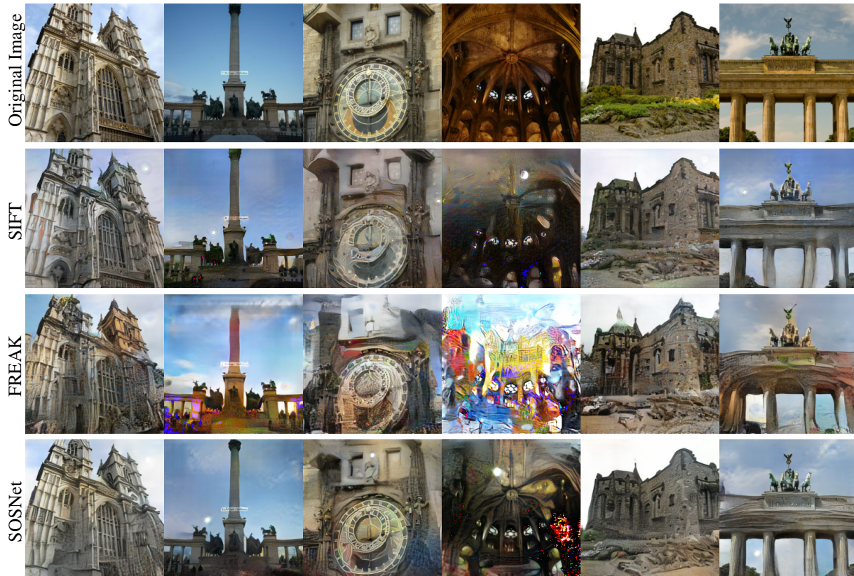
Figure 3: Reverse Engineering Attack Results. From top to bottom: ground truth and reconstructions from a max. of 1,000 sparse SIFT, FREAK and SOSNet features. One can observe that reconstruction from only sparse local features reveals the original image information extremely well. Note that the images show landmarks that were not included in the training data.
