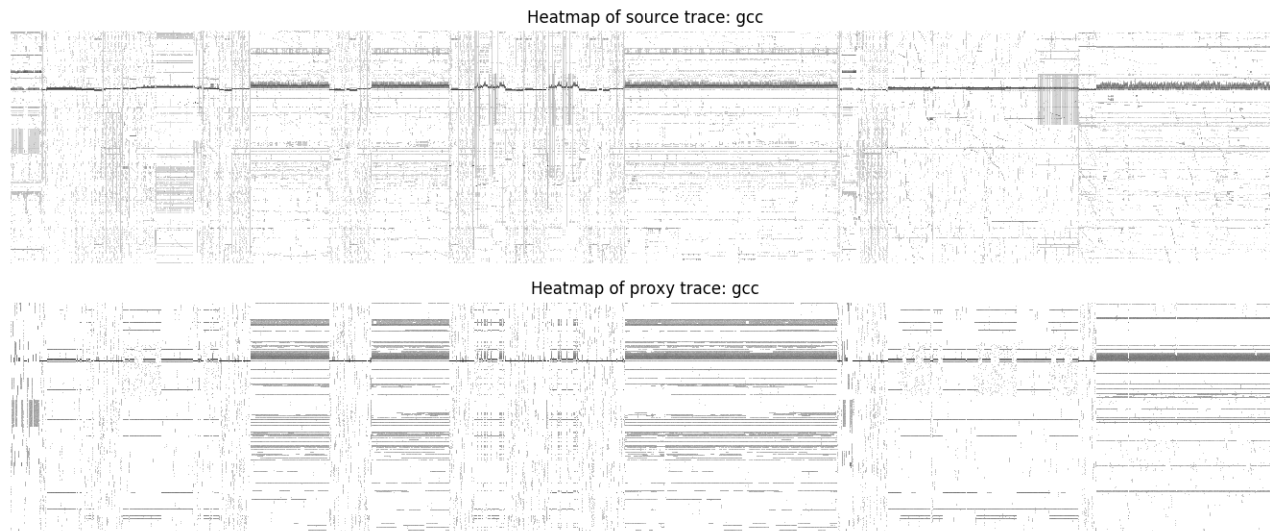
Figure 7. Heatmap for the original gcc trace and the trace-wrung proxy generated for gcc trace from the wrapped address space. Each pixel corresponds to one wrapped address at one time step. The darker the pixel, the more times that address is accessed during that time step.
